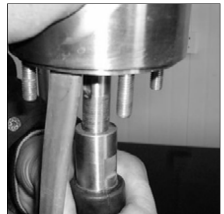
Figure 14: Assembling the Rotor on the Motor Shaft
